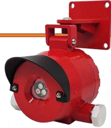
The detectors uses 3 infrared sensors with different wavelengths with narrow-band filtering. One sensor is used to reflect the centre wavelength of the flame information. The other sensor is used to monitor other infrared radiation in the environment. Combining with the flicker characteristics of the flame, analyzing through high-speed microprocessors and circulating by mathematical algorithms, the radiation spectrum with flame characteristics is confirmed as a fire alarm.
